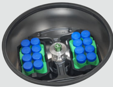
H-Flex 1 Swinging Bucket Rotor, 90°, R max 170 mm
